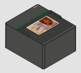
Afterwards, the ID card, passport or driver's license are placed on the scan window to compare the captured certificate data with the data on the ID document.
